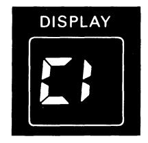
This flashing code tells you to check the automatic icemaker. Ice clumps in the storage bin may have stalled the icemaker. Follow corrective measures described on page 12. If water supply to the icemaker is not connected or not turned on, make sure manual icemaker switch is in the OFF position (see page 10). Code stops flashing when problem is corrected or STATUS CHECK-RESET pad is touched.
